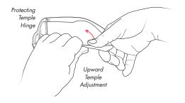
Grasp the temple arm with one hand at mid length to isolate any movement that can stress the hinge.
