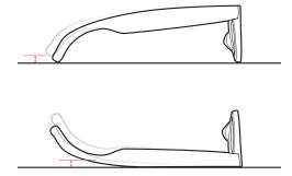
Placeyourglassesonaflatsurfacetoensure level alignment. Both temples should touch the surface on the same plane.
