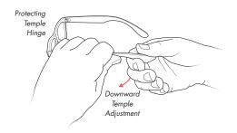
Grasp the temple arm with one hand at mid length to isolate any movement that can stress the hinge.
